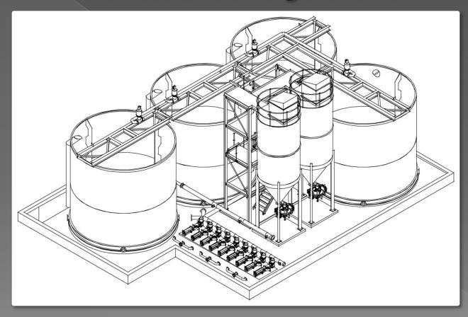
High Capacity C-250 Flocculant Plant with twin 20 ton storage silos and duel high energy hydrators. Plant is shown with 4 X 175 cubic meter tanks.
