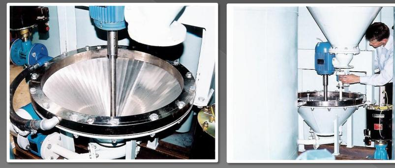
The RESOURCES<sup>IM</sup> proprietary High Energy Pump Hydrator ensures an even and complete water coating of the individual reagent particles, eliminating clotting. The water pressurized annular ring creates an even water curtain over the entire hydrator surface with no dry areas. A high energy pump then transfers the initially wetted reagent to the hydration tanks.
