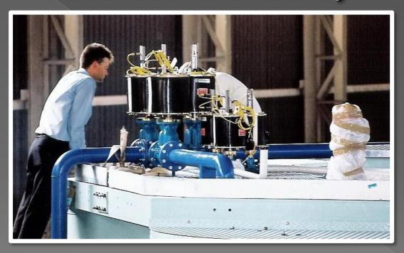
The Pneumatic Main Water Distribution Valve Assembly is used for filling of the primary sequence tanks. The larger main water distribution valves are used to achieve rapid filling of the tanks. The smaller wetted flocculant distribution valves are used to introduce the wetted flocculant from the hydrator to the appropriate sequence tank. The compact single point location of the valves allows easy inspection and maintenance.
