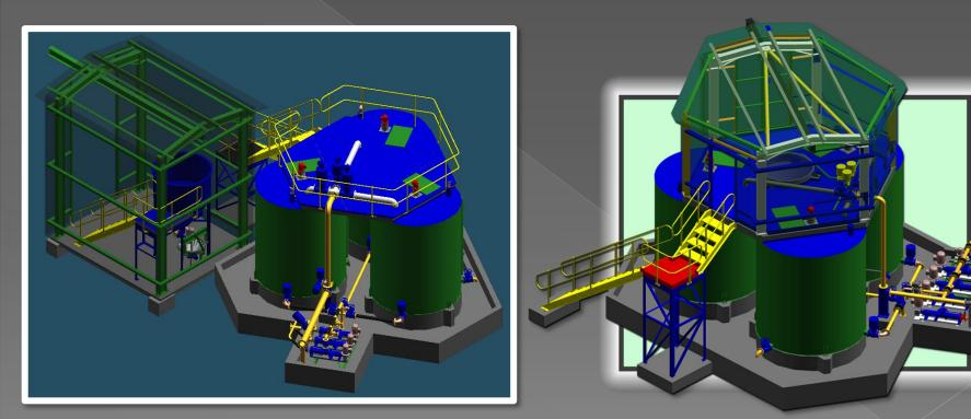
Extended configuration with flocculant handling separate from tanks
