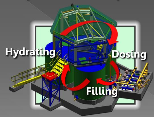
**Sequencing Control Strategy:** Each of the tanks sequentially rotate in their function. At any given time, one tank will be dosing correctly hydrated polymer to the process, while the other tanks will be performing hydrating and filling functions respectively.
