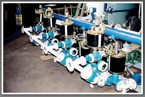
The Dilution Assembly is for dilution to process concentration. Delivery lines are equipped with flow measurement to ensure continuous accurate dilution ratios under all operating conditions. This automation allows multiple pumps to independently operate at whatever delivery rate is required for correct concentration to numerous delivery points.
