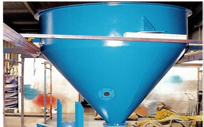
**Steep Angled Hopper-** eliminates dry reagent bridging and material flow hindrance. Inner surface of hopper is coated with specialized ultra low friction coating for smooth movement of dry material. Air inlet flange and fluidizing air piping is provided should this be required for certain flocculants.
