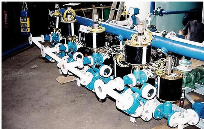
**Dilution Assembly-** for dilution to process concentration. Delivery lines are equipped with flow measurement, to ensure continuous accurate dilution ratios under all operating conditions. This automation allows multiple pumps to independently operate at whatever delivery rate is required for correct concentration to numerous delivery points.
