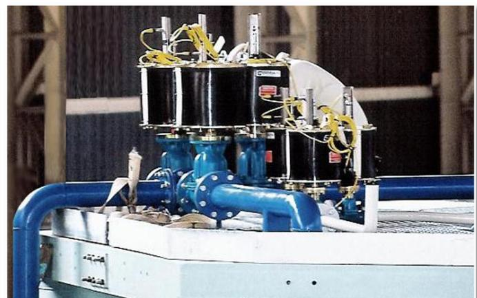
**Pneumatic Main Water Distribution Valve Assembly-** for filling of the primary sequence tanks. Compact single point location for ease of maintenance. All automatic valves are equipped with proximity sensors for position status confirmation.
